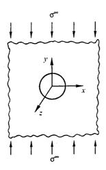
Figure 1: Panels weakened by hole in compression
