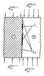
Figure 5: Model for fracture investigations of the vicinity of point A at the second level of analysis
