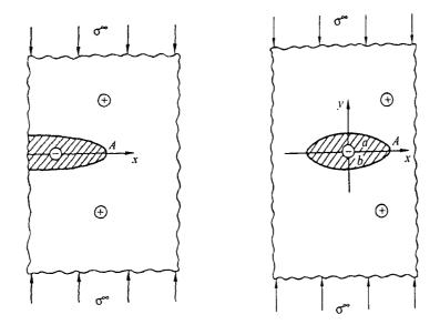
Figure 3: Crack-tip vicinity in case of filled crack
