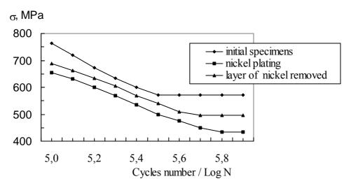
Fig.5. Curves of fatigue of specimens after electrochemical nickel plating.
