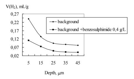
Fig. 4. Distribution of hydrogen across of steel base after electrochemical nickel plating 20  $\mu$ m thick.
