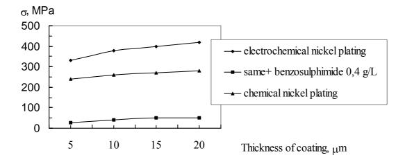
Fig. 2. Residual stresses in nickel coating.
