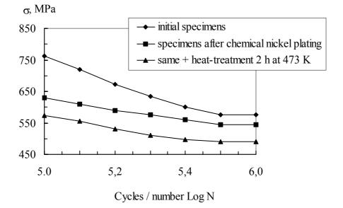
Fig. 3. Curves of fatigue of specimens after chemical nickel plating.
