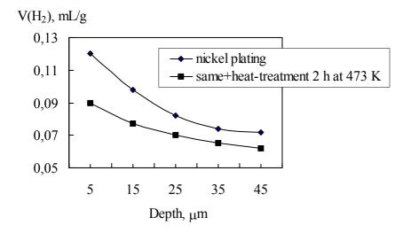
Fig.1. Distribution of hydrogen across of surface layer of the steel base after chemical nickel plating 20  $\mu$ m thick.
