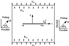
Fig.1 Crack in magnetoelectroelastic material.
