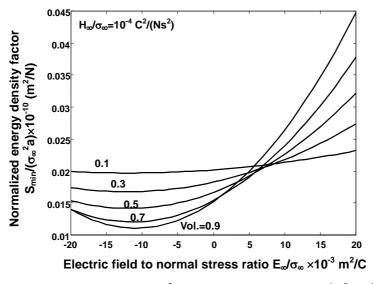
Fig. 3. Normalized  $S_{min}/\sigma_{\infty}^2$  a with  $E_{\infty}/\sigma_{\infty}$  for  $H_{\infty}/\sigma_{\infty} = 10^{-4} C^2/(Ns^2)$ .
