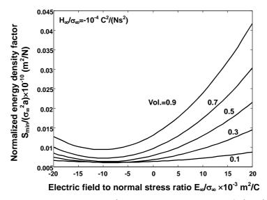
Fig. 2. Normalized  $S_{min}/\sigma_{\infty}^2 a$  with  $E_{\infty}/\sigma_{\infty}$  for  $H_{\infty}/\sigma_{\infty} = -10^{-4} C^2/(Ns^2)$ .
