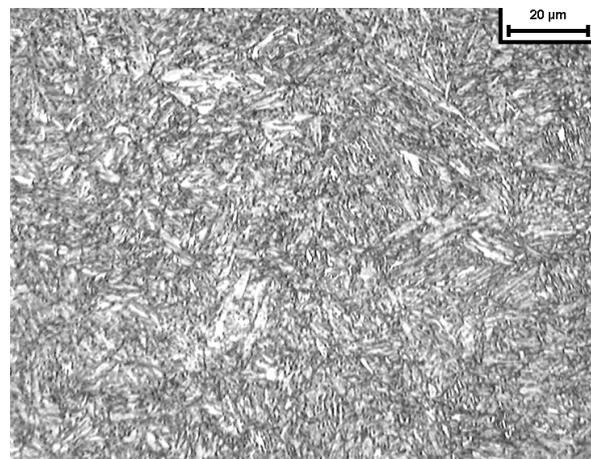
Fig. 3 – O1 blank microstructures at different distances from the bloom surface: (a) 149 mm, tempered martensite and bainite; (b) 280 mm, tempered martensite and bainite with pearlite and some ferrite appearing at prior austenite grain boundaries. 1% Nital etch.
