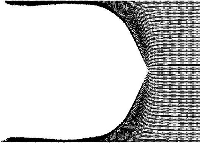
Figure 2: Supersonic crack in Mooney-Rivlin rubber, studied with the method of multi-particle modeling described above. Parameters are chosen to match the experiments in [1, 2]
