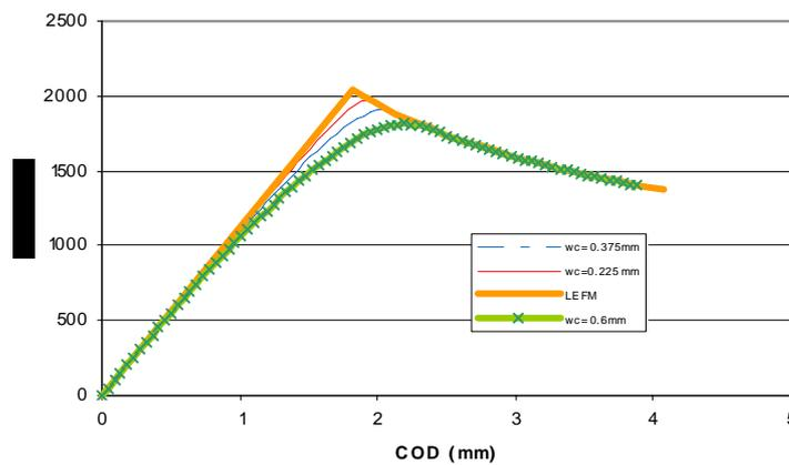
Figure 2 : Force-COD curves obtained by NLFM and LEFM FE-Simulations
