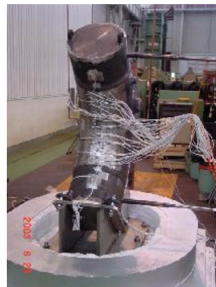
Fig.1 Appearance of the elbow at the burst test stand
