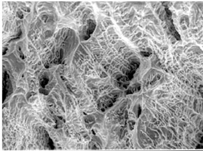
Fig. 3 Fractograph of 6 wt.% quartz chilled MMC (Magnification 100  $\times$ m)
