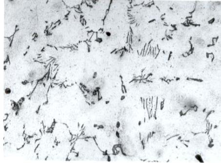
Fig. 2 Microstructure of 9 wt.% quartz chilled MMC.(Magnification 500 X)
