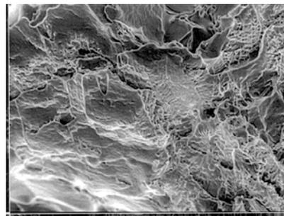
Fig.4 Fractograph of 9 wt.% quartz chilled MMC (Magnification 100  $\times$ m)
