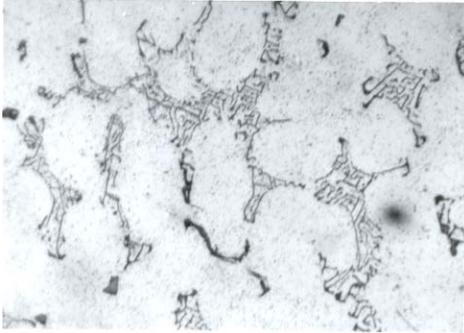
Fig. 1 Microstructure of 6 wt.% quartz chilled MMC (Magnification 500 X)
