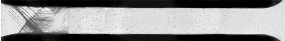
Figure 4: Optical images of the surface of the armco-iron specimen subjected to equal-channel angular pressing with subsequent annealing at 623 K,  $\epsilon=7\%$  [5]
