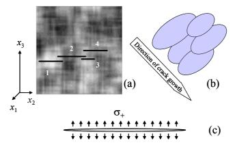
Figure 1: Macroscopic crack formation and growth under spatially random stress field: (a) a realisation of the random stress field  $\sigma_{33}$ ; the maximum compression is shown in black, the tension - in white. The first crack segment (crack 1) appears at the place of maximum tension. Crack 2 is then generated at the place where the compressive stress is minimal, then other segments (cracks 3 and 4) are generated; (b) a 3D structure of the macrocrack; (c) a model of the macrocrack.
