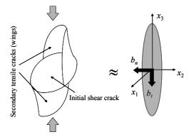
Figure 2: Wing crack evolved form an initial inclined shear crack (left) and its model as a dislocation loop (right) with Burgers vector  $(b_t, b_n)$ .
