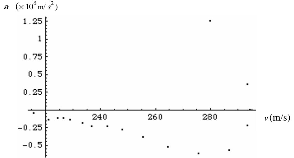
Fig. 1 The crack acceleration versus the velocity of the crack for PMMA
