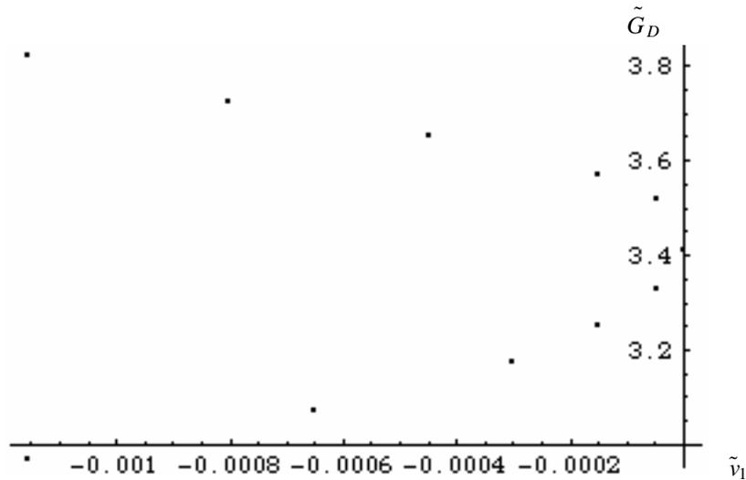
Fig. 2 The normalized fracture toughness versus the normalized velocity of the crack for PMMA
