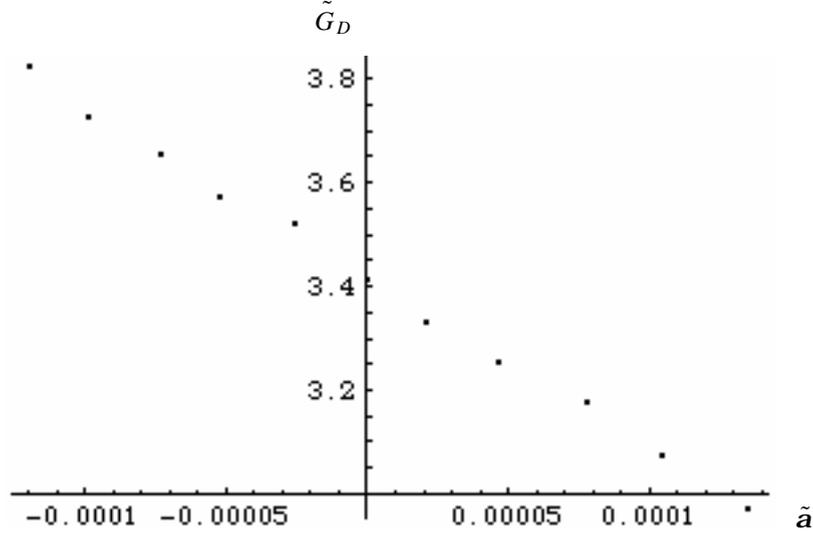
Fig. 3 The normalized fracture toughness versus the normalized crack acceleration for PMMA
