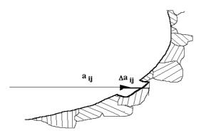
Figure 1: Microstructural configuration at the crack front: The crack front cuts many grains with different orientations and grain length; the crack is moving in one crack front segment  $a_{ii}$  by  $\Delta a_{ii}$ .
