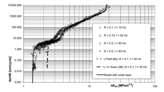
Figure 3: Fitted Probability Functions and Crack Growth Rate Data for 7075-T651 in air
