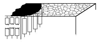
Figure 2: Micromechanical configuration at the crack front and the modeling with single elements
