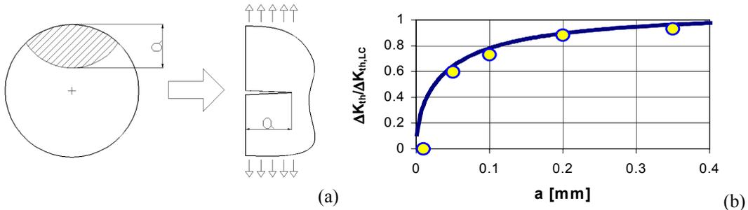
Fig.5: Threshold for short cracks: a) equivalence between elliptical crack and surface crack; b) Kitagawa diagram for surface crack.
