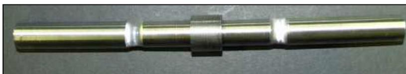
Fig.1: The small scale specimen with a press-fitted cylinder.
