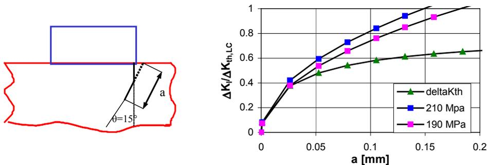
Fig.9: Determination of fatigue limit for 3D specimen.
