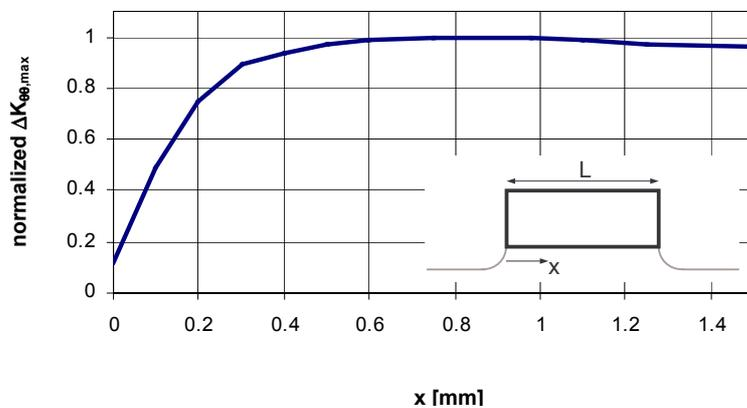
Fig.8: Calculation of  $\Delta K_{\theta\theta, \text{max}}$  for a prospective crack along the contact edge.
