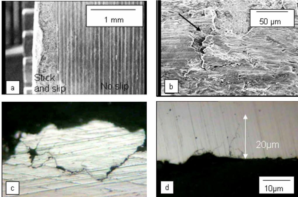
Fig.3: Fractographic observations: a) surface damage near fracture surface; b) fretting scars; c and d) non propagating cracks observed on polished sections.
