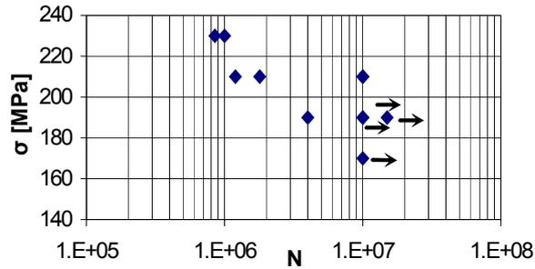
Fig.2: S-N diagram for 3D fretting specimens..
