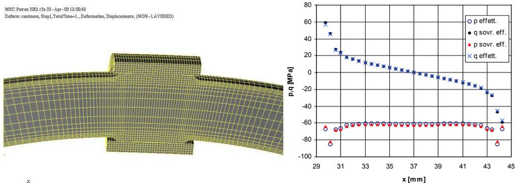
Fig.6: FE analysis: a) 3D specimen finite element model; b) surface contact stresses.
