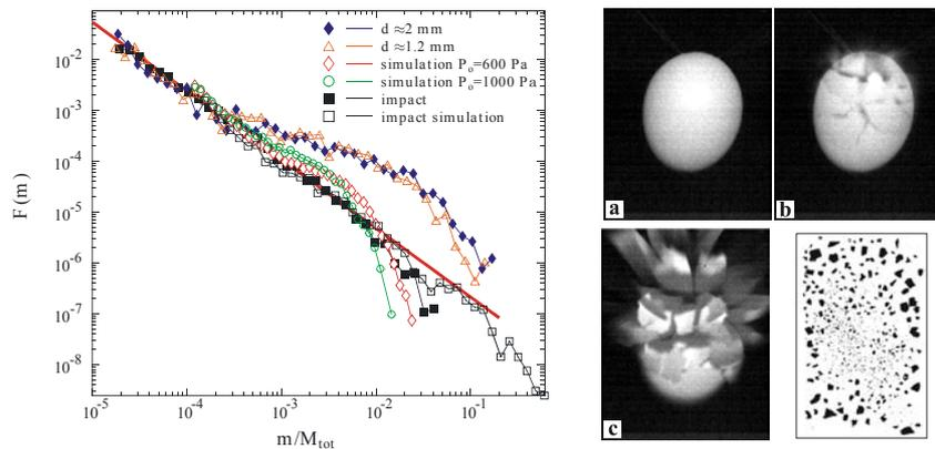
Figure 2: Comparison of fragment mass distributions obtained by explosion experiments with two different sizes of holes and a-c) impact experiments with results of the simulation and time evolution of the explosion of an egg taken by a high speed camera with 1kHz.
