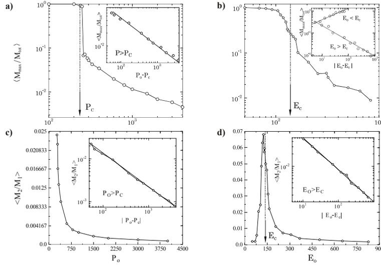
Figure 4: Average mass of largest, and second largest Fragments (a,b) and average fragment mass (c,d) as functions of control parameters,  $P_0$  and  $E_0$
