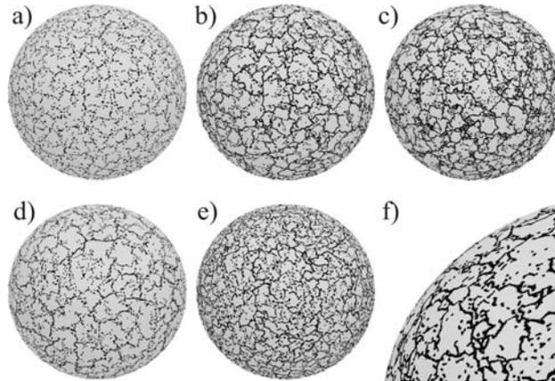
Figure 3: The time evolution of the breakup process under a constant pressure of  $P_0/P_c \approx 4.0$  a-c), until the final state c) is reached with a magnified view f). Final states of impact simulations are shown for energies  $E_0/E_c \approx 0.8$  and  $2.8$  d),e). Particle positions are projected on their initial positions. Fragments are identified as shell pieces surrounded by cracks.
