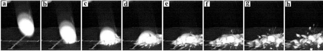
Figure 1: Time series of the gradual collapse of an egg shell due to impact with the hard ground.
