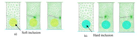
Figure 4. Crack propagation in a part with a) a soft inclusion R=10, b) a hard inclusion R=0.1
