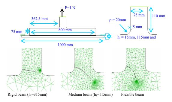
Figure 3. Crack growth from a fillet and influence of the support beam rigidity on the crack path.
