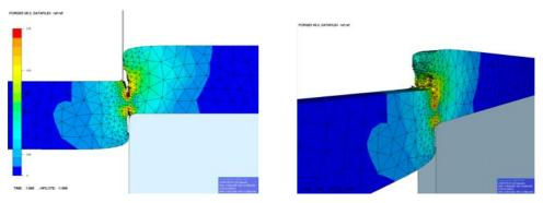
Figure 1. Blanking simulation: isovalues of damage during fracture
