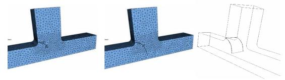
Figure 5. 3D crack growth from a fillet
