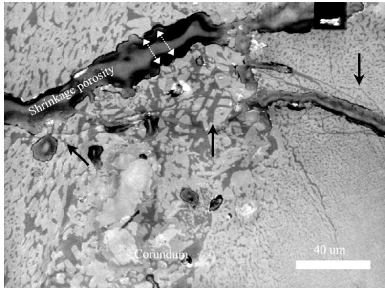
*Fig. 2: Example of thermoshock-induced microcrack splay (arrows) relieving stresses between open elongated pores but refilled by melt (healed) during a subsequent thermal equilibration cycle. Note net dilatation of segmented individual mullite microcrystals. Reflected Light, glass is darker grey.*
