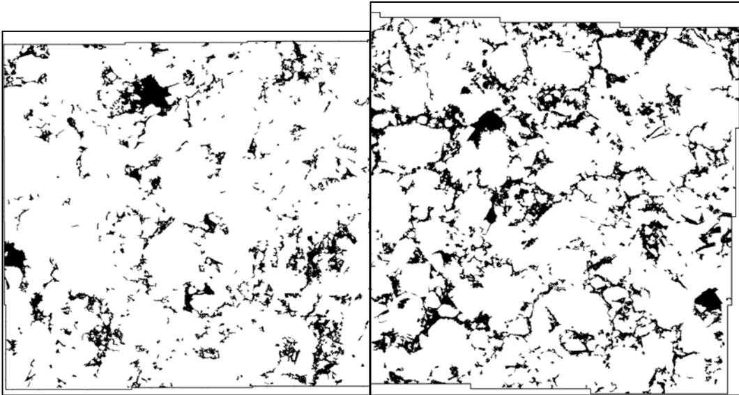
*Fig. 3: Tracing of connected porosity (black) from image analysis. View onto the surface of the discs. Left: Original material; Right: After 6 downquench shocks from 1300 °C. Each image is 11 mm wide. Area fraction of connected porosity is 9.8 % in the left image, 13.2 % in the right image. Note the increase in connectivity of large pore complexes in the after-shock image.*
