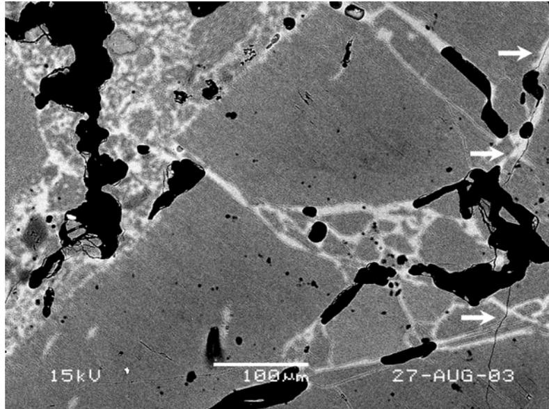
*Fig. 1: (SEM image) Example of the general refractory microstructure: note the distinction between a blocky mullite glass symplectite pseudomorphs after original andalusite and intergranular crystal-melt mush (ceramic bond; melt is light-grey). Note the presence of porosity connected with extensive melt filled pre-thermoshock fractures. Arrows indicate a thermoshock-derived fracture connecting pre-existing porosity with disregard to melt or mullite.*
