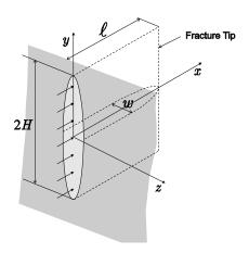
Figure 1: Schematic of the PKN hydraulic fracture model.
