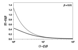
Figure 3: Plot of normalized correction  $|\Pi - \Omega|/\beta$  versus normalized distance from the tip  $(1 - \xi)/\beta$ . Comparison of numerical results (dots) versus outer expansion (solid line). Results obtained using  $\Omega = (1 - \xi^2)^{2/3}$  and  $\beta = 0.01$ .
