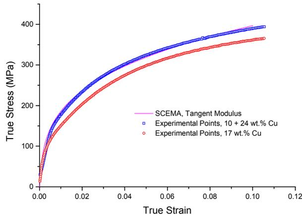
Figure 2: The compressive stress-curve is plotted for two Al-17wt%Cu alloys – one with a uniform distribution of  $\text{CuAl}_2$  (lower data) and the other with a clustered distribution (upper data). The solid line represents the predicted curve for the bimodal distribution derived from a self-consistent analysis using the flow curves of uniform composites containing 10 and 24wt% Cu as input.
