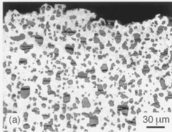
Figure 1: Damaged (cracked) particles near the fracture surface of an Al-20%Si alloy. The particles are essentially pure silicon [12].
