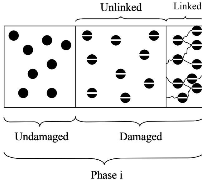
Figure 3: Conceptual illustration of the progressive linkage of cracks in the damaged region of the concept as described by the micro-crack linkage model. Each “phase” obeys a somewhat different constitutive behaviour which recognizes the effect of particle cracking and damage linkage on the strength of the composite.
