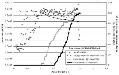
Fig. 3: Experimental data: Youngs modulus reduction, crack densities and acoustic emission data as a function of axial strain
