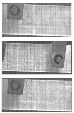
Fig. 2: Matrix cracking failure modes: transverse cracking, splitting and debonding of the stitching yarns
