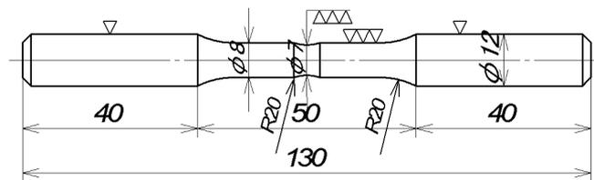
Figure 3. Shape and size of fatigue test specimen. unit:mm
