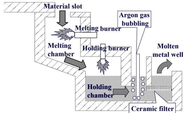
Figure 2. Schematic degassing process system.
