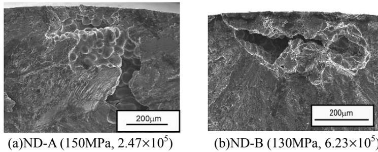
Figure 7. Crack initiation sites of ND materials.
