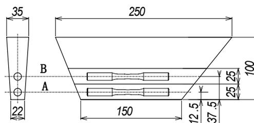
Figure 1. Extracted position of specimens.
