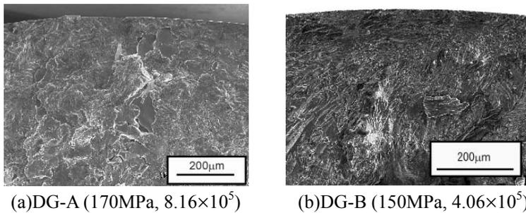
Figure 8. Crack initiation sites of DG materials.
