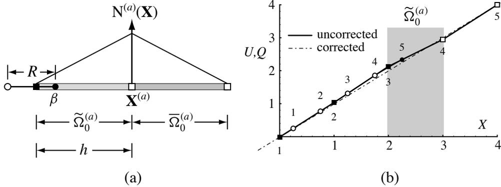
Figure 2: (a) Patch from a 1-dimensional coupled system. (b) Displacements of the 1-D coupled system for both the corrected and uncorrected bond density. Atom and node numbers are shown.
