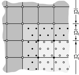
Figure 1: Patch of a coupled atomistic-continuum system. The set of FE nodes  $\mathcal{N}$  is shown as open squares  $\square$ . The set of nodes  $\hat{\mathcal{N}}$  is shown as solid squares  $\blacksquare$ . The set of atoms  $\mathcal{A}$  is shown as open circles  $\circ$ , and the set of atoms  $\hat{\mathcal{A}}$  is shown as solid circles  $\bullet$ .
