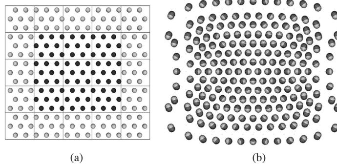
Figure 3: (a) A 2-D, triangular lattice with free surfaces composed of free (light grey) and ghost (dark grey) atoms. (b) The relaxed configuration of (a) for the coupled system (dark grey) and a system treated purely with atomistics (light grey). Displacements are magnified by a factor of 200.
