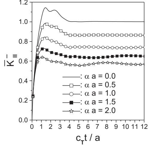
Fig. 5:  $\bar{K}_{II}^-(t)$  versus dimensionless time
