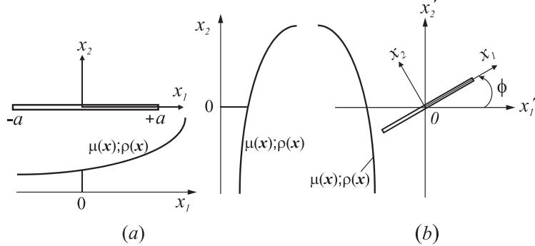
Fig. 1: An infinite FGM containing a finite crack
