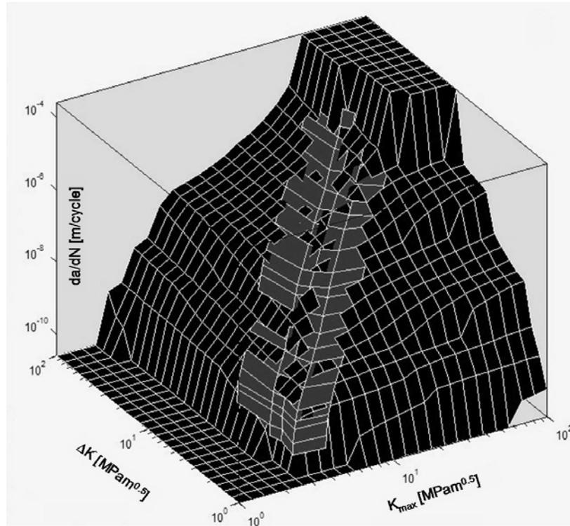
Fig. 3 Fatigue crack growth data [12] of 7055-T7511 aluminum alloy as a function of  $\Delta K$  and  $K_{\max}$ .
