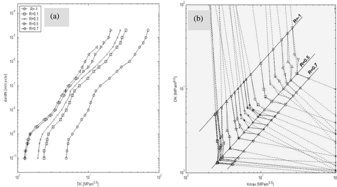
Fig. 2 Fatigue crack growth data [12] of 7055-T7511 aluminum alloy as a function of (a)  $\Delta K$  and (b)  $\Delta K$  and  $K_{max}$  for constant  $da/dn$ .
