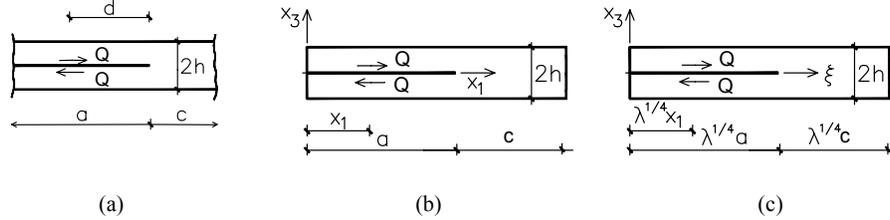
Figure 2: (a) infinite strip with semi-infinite crack loaded in mode II; (b) double cantilever beam loaded in mode II by pair of tangential forces  $Q_i$  acting at the coordinate  $x_{1i}$ ; (c) rescaled problem
