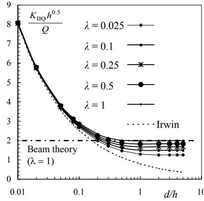
Figure 3: dimensionless stress intensity factor in a degenerate orthotropic double cantilever beam loaded in mode II. Influence of  $\lambda$  on the solution.
