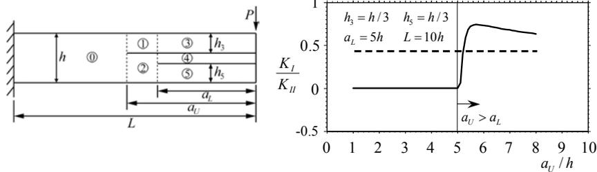
Figure 1: (a) cantilever beam with multiple delaminations; (b) influence of the interaction between delaminations on the mode ratio in a multiply delaminated beam.
