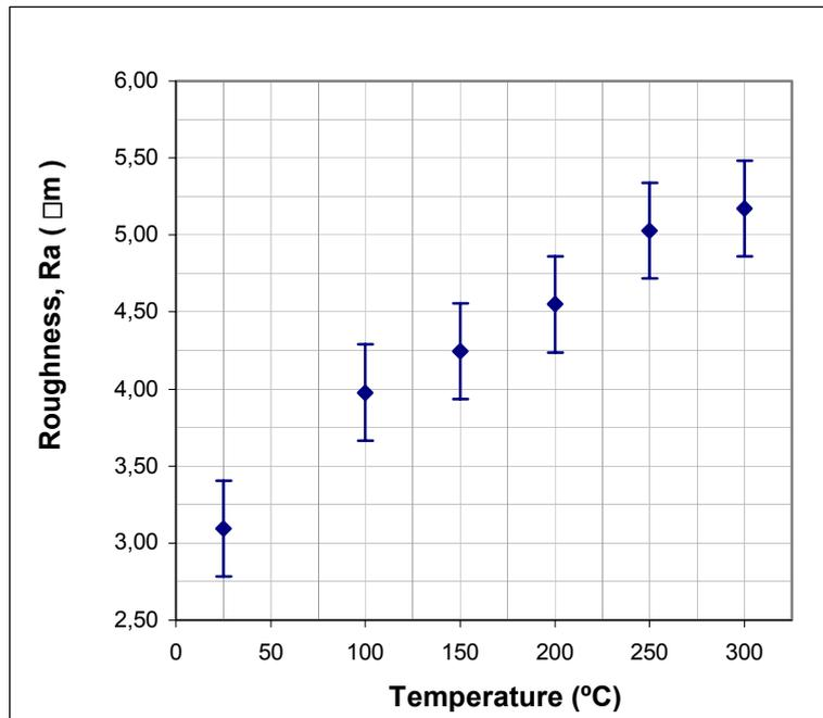
Figure 2: Roughness, measured in terms of Ra, as function of the shot peening temperature.
