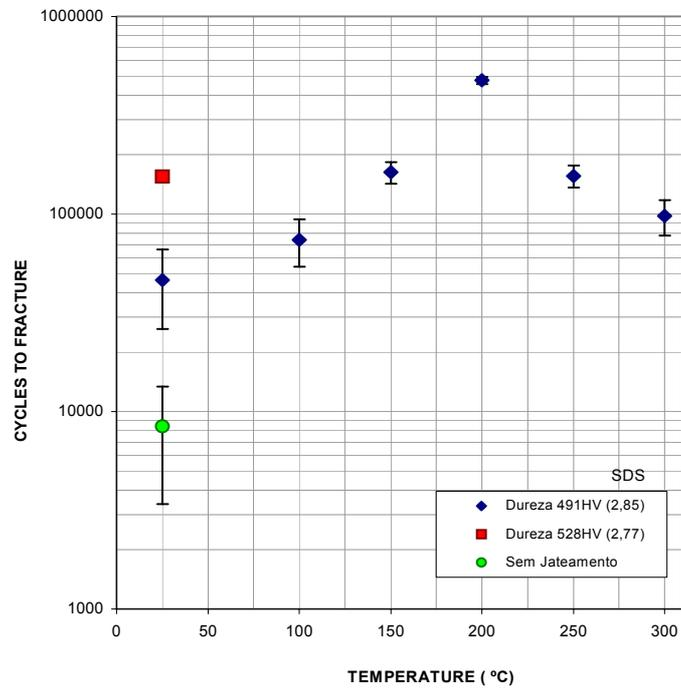
Figure 1. Mean fatigue life versus shot peening temperature.
