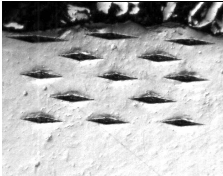
Figure 4. Knoop microhardness indentation close to the shot peened surface.
