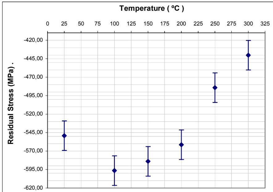
Figure 3. Residual stress mean value versus temperature of shot peening.
