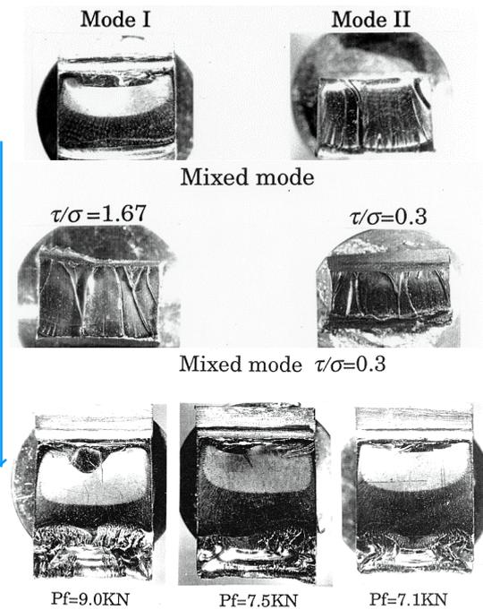
Fig. 5. Optical photographs of the fracture surface for mode I, mode II and mixed mode. Arrow indicates crack propagation direction
