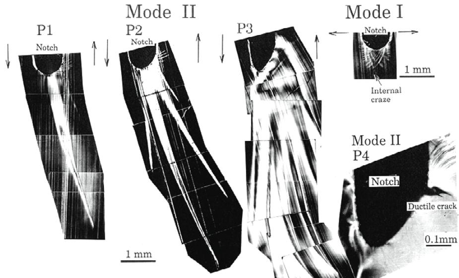
Fig. 3 Polarized micrographs of thin sections of the local deformation region ahead of notch for mode I and mode II loading
