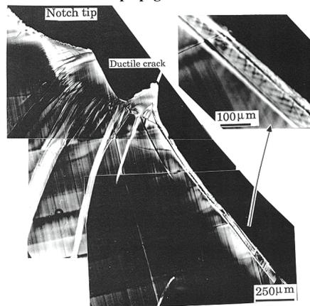
Fig.7 Polarized micrographs of a thinned section of the fracture subsurface of Fig.6.
