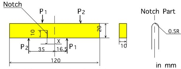
Fig. 1 Shape and dimensions of test specimens
