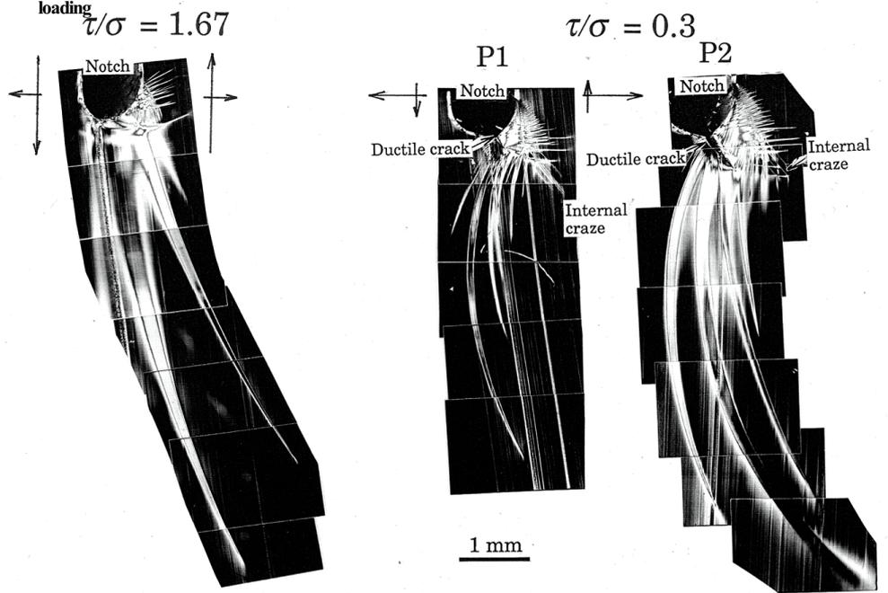
Fig. 4 Polarized micrographs of thin sections of the local deformation region ahead of notch for mixed mode loading
