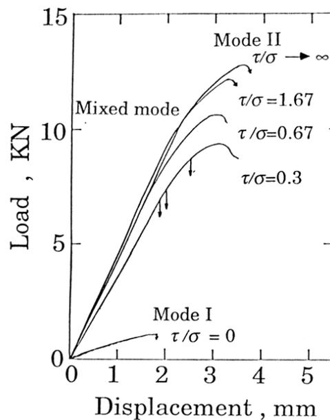
Fig. 2 Typical load-displacement curves of PC under mode I, mode II and mixed mode
