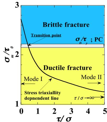
Fig.8 Stress triaxiality dependence of applied stress components ratio.
