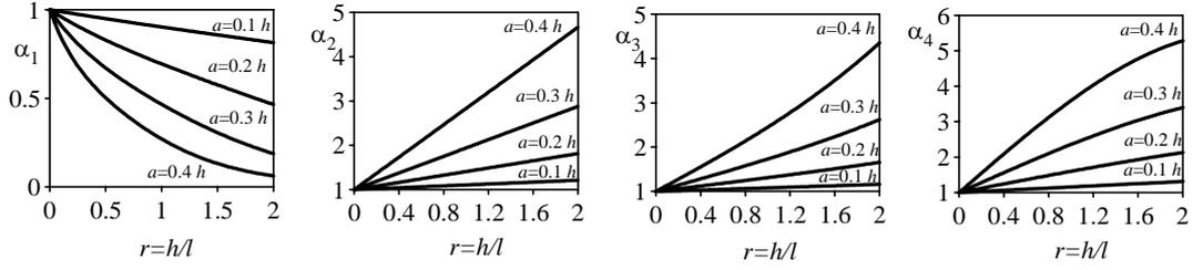
Figure 1: Coefficient values in the stiffness matrix of the cracked element ( $r = h/l$  is the ratio between the height and the length of the element;  $a$  is depth of the crack).
