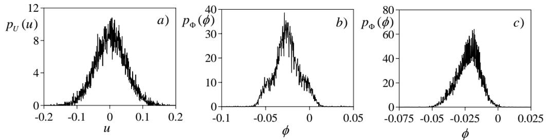
Figure 4: probability density functions of the response process: a) displacement at restraint (input signal); b) rotation below the crack; c) rotation above the crack
