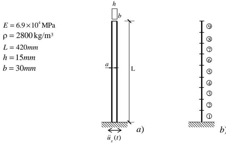
Figure 2: Cantilever beam (a) and finite elements model (b)
