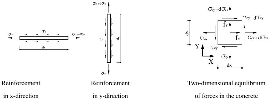
Figure 4 Two-dimensional equilibrium of forces in the reinforcing bars and concrete
