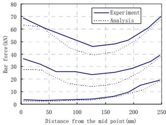
Figure 8. Comparison of bar forces between experiment and analysis
