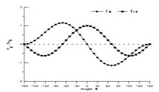
Figure.2 Angular variation of circumferential  $f_{\theta}$  and shear  $f_{r\theta}$  in pure shear loading
