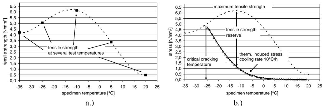
Figure 6: Testing of AB 11: (a) UTST and (b) comparison between TSRST and UTST results.
