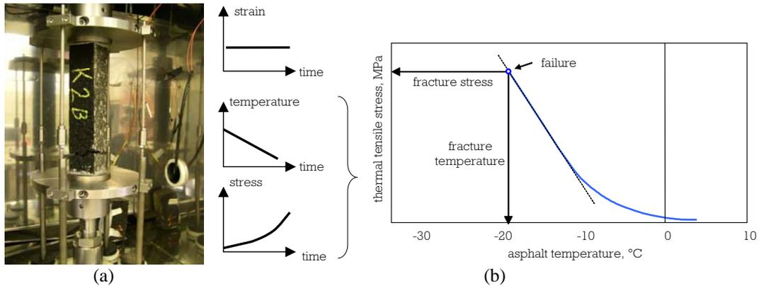
Figure 3: TSRST: (a) experimental setup and (b) illustration of result from TSRST.
