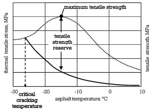
Figure 2: Superposition – tensile strength reserve.
