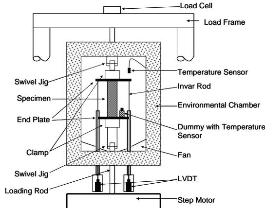
Figure 4: Illustration of setup of the employed testing equipment at the Christian-Doppler Laboratory.
