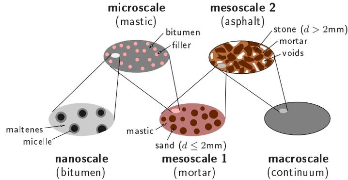
Figure 1: Multiscale model for asphalt comprising five scales of observation [2].
