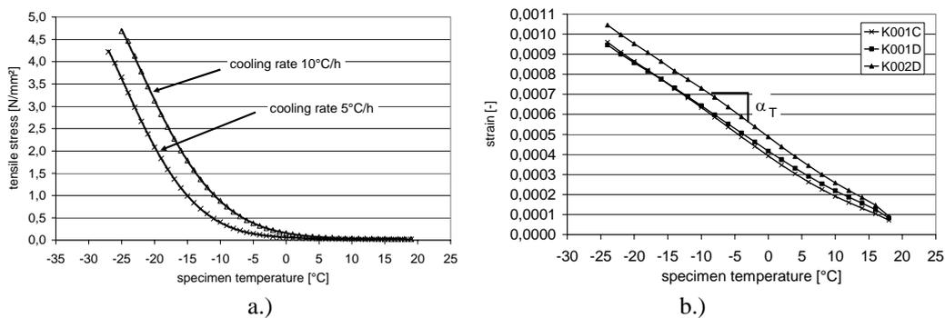
Figure 5: Results from testing of AB 11: (a) TSRST and (b) shrinkage test to derive  $\alpha_T$ .
