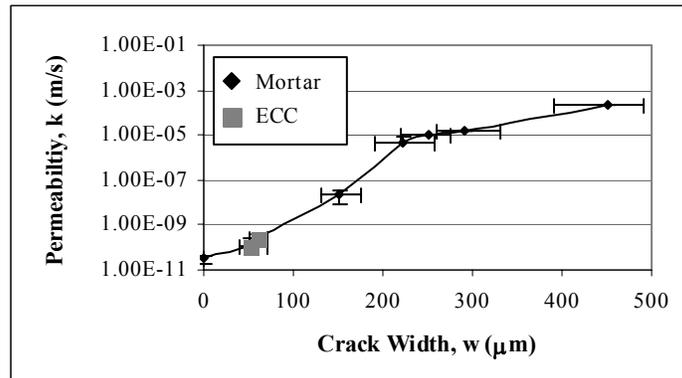
Figure 5: Water Permeability of Cracked ECC and Concrete (See Table 2 for crack widths)
