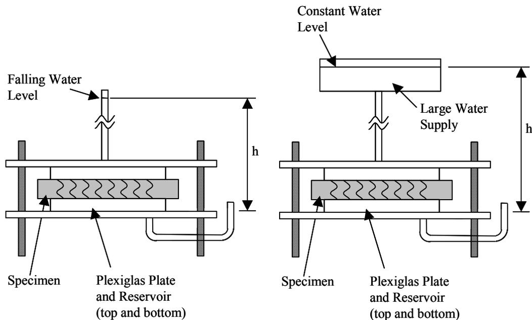
Figure 3: Falling Head Test
