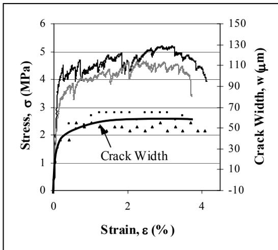
Figure 1: ECC Tensile Stress-Strain Response
