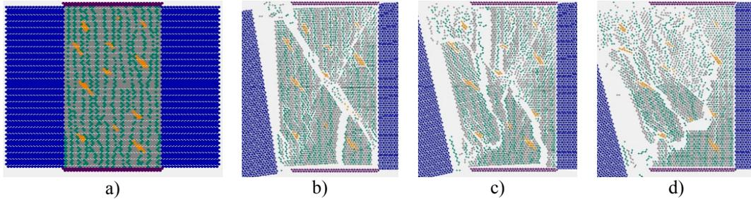
Figure 2: Initial structure of the set-up (a) and fracture patterns of the fine detritus specimen after left wall freeing ( $\varepsilon_v=2.75\%$ ): b)  $E_s=0.3 \times E_{fD}$ ; c)  $E_s=E_{fD}$ ; d)  $E_s=3 \times E_{fD}$ .
