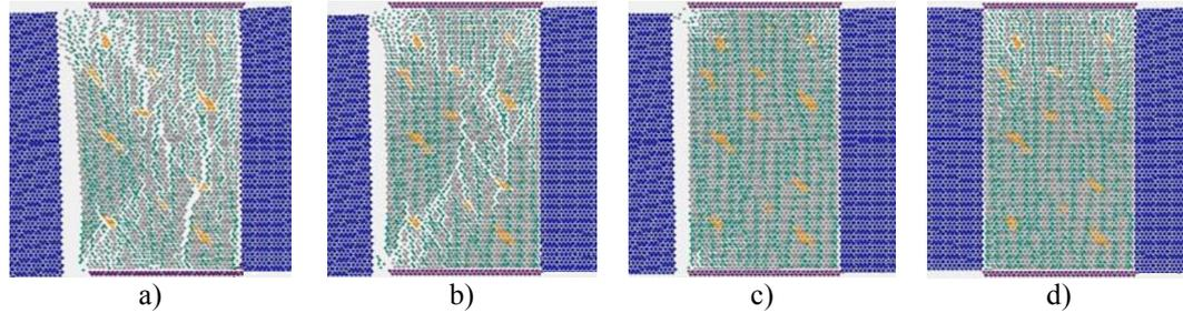
Figure 3: Fracture patterns of the fine detritus specimen after left wall freeing ( $\sigma_v=16$ MPa): a)  $E_s=0.33 \times E_{fD}$ ; b)  $E_s=E_{fD}$ ; c)  $E_s=3 \times E_{fD}$ ; d)  $E_s=E_{fD}$  (another procedure).
