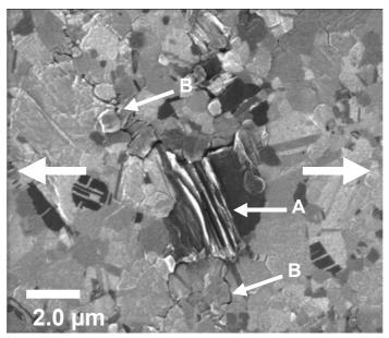
Fig. 1: FIB planview micrograph of a 3  $\mu$ m thick Cu film after a fatigue experiment with a total strain range of about 1% showing an extrusion (A) and cracks (B). The loading direction was horizontal.
