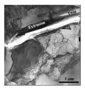
Fig. 3: TEM micrograph of a 400 nm thick Cu film after a fatigue experiment with a total strain range of about 1% showing an extrusion at the surface and crack extending across the entire grain (from [6]).
