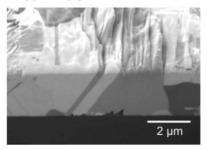
Fig. 2: FIB cross-sectional micrograph of a 3  $\mu$ m thick Cu film after a fatigue experiment with a total strain range of about 1% showing an extrusion at the surface and voiding near the interface. The loading direction was horizontal.
