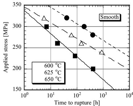
Fig.1 Relationship between time to rupture and applied stress under uni-axial creep tests
