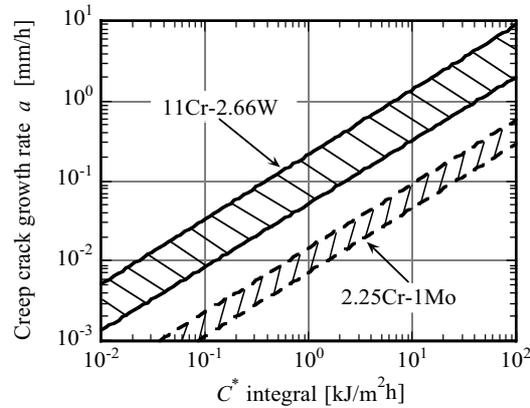
Fig.9 Comparison of creep crack growth property between 11Cr-2.66W and 2.25Cr-1Mo steels
