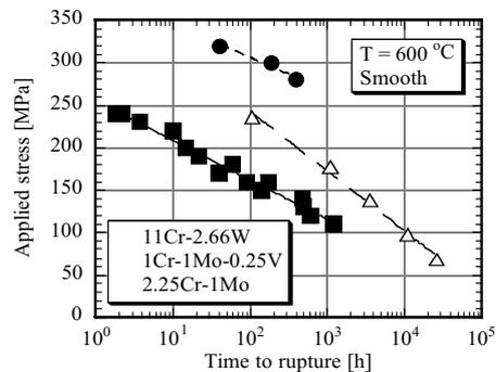
Fig. 2 Comparison of time to rupture with other heat resistant materials
