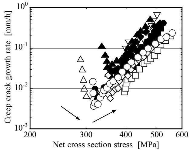
Fig.7 Evaluation of the creep crack growth rate on net cross section stress. Symbols means the same in Fig.8.
