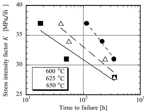
Fig.5 Relationship between time to failure and stress intensity factor in creep crack growth tests.
