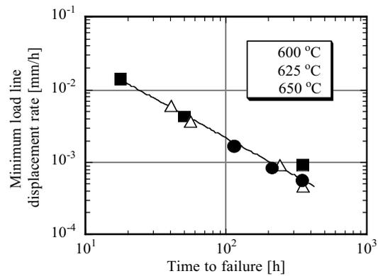
Fig.6 Relationship between time to failure and minimum loadline displacement rate in creep crack growth tests.
