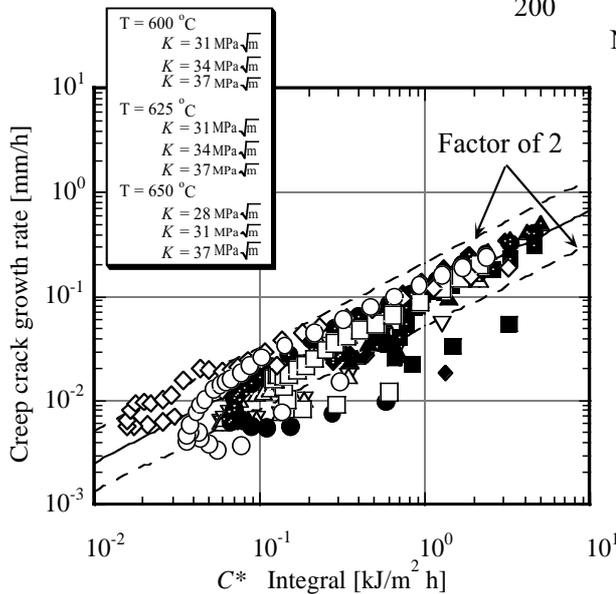
Fig.8 Relationship between creep crack growth rate and  $C^*$  parameter.
