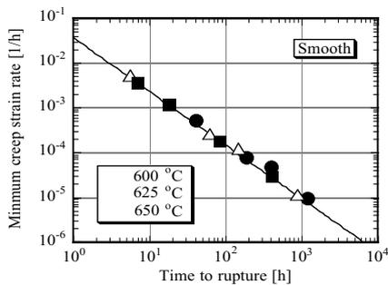
Fig.3 Relationship between time to rupture and minimum creep strain rate under uni-axial creep tests
