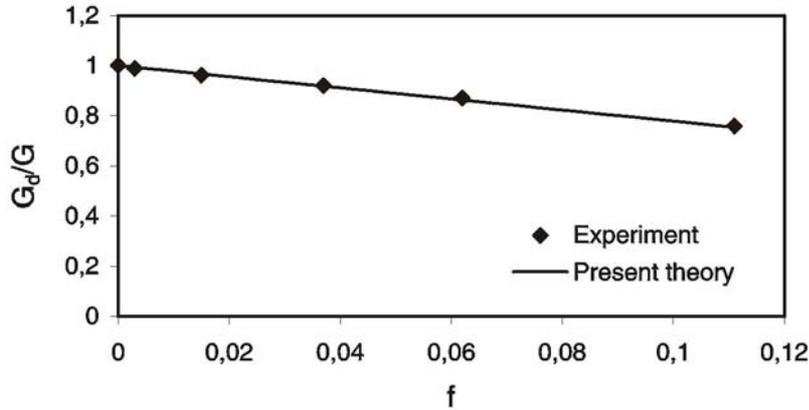
Figure 1: Effect of porosity on the shear modulus.
