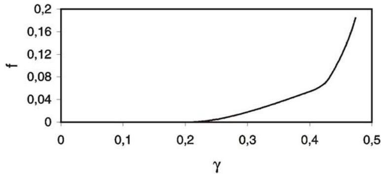
Figure 3: Current void volume fraction vs. equivalent plastic strain.
