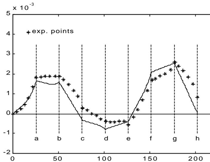
Figure 2: Comparison of the theoretical and experimental strain responses in the  $x_3$  direction (the abscissa numbers correspond to the steps of absolute values of stress used in the calculation)
