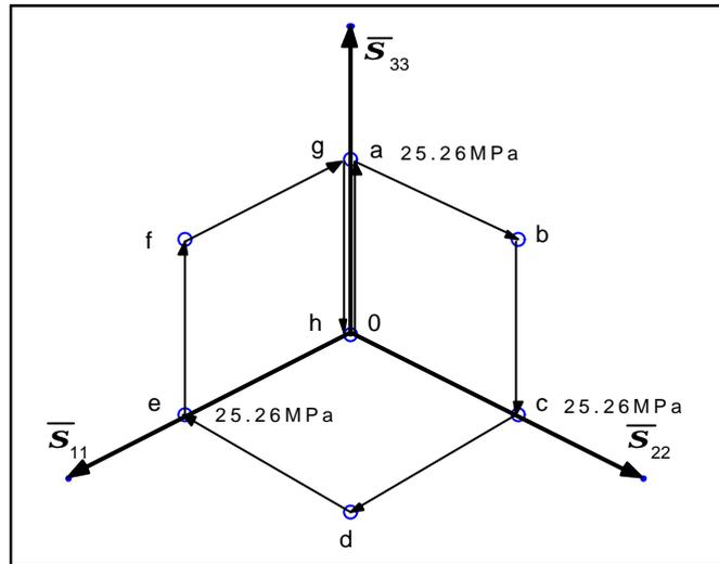
Figure 1: The complex loading path under investigation – a sequence of compressive loading processes in three orthogonal directions.
