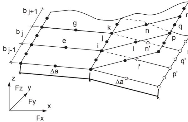
Figure 4: Model with 8-noded shell element near the debonding front.
