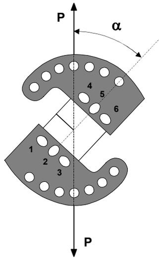
Figure 1: Loading of the CTS specimen.
