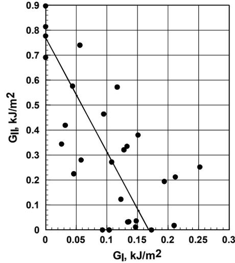
Figure 2: Approximation of mixed mode experimental data for eqn (3).
