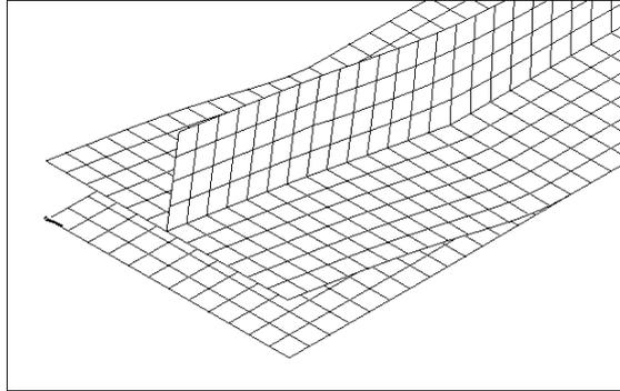
Figure 3: Finite element mesh of the skin-stringer deformed model.
