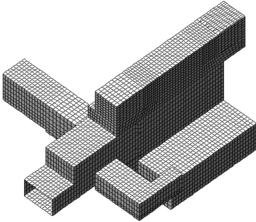
**Figure 2:** Finite element model of zone 1
