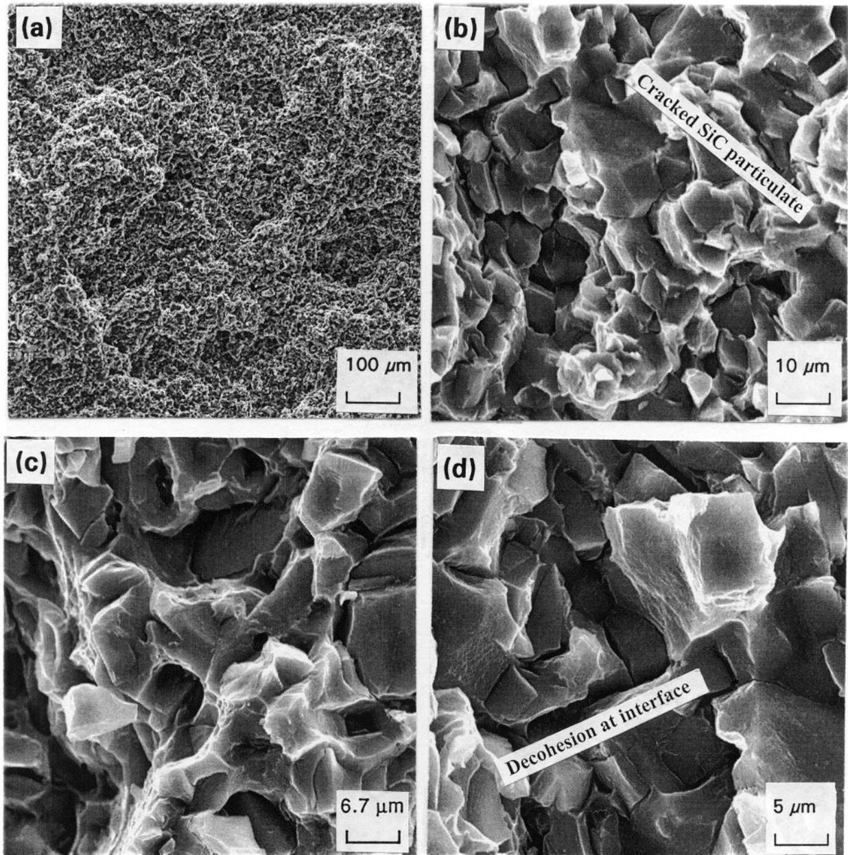
Figure 2. Scanning electron micrographs of the 7034/SiC/15p-UA composite deformed at 27°C and showing the following features: (a) overall morphology, (b) tear ridges, (c) cracked SiC particulates and decohesion at matrix-particulate interfaces, (d) microscopic features of fracture at the higher test temperature (120°C).
