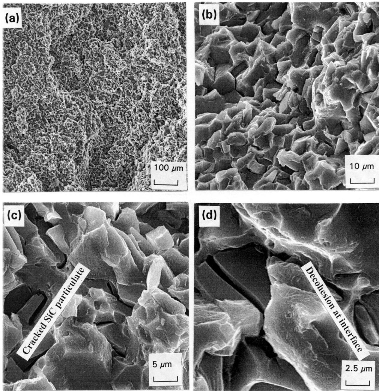
Figure 3. Scanning electron micrographs of the 7034/SiC/15p-PA composite deformed at 27°C and showing the following features: (a) overall morphology, (b) tear ridges, (c) cracked SiC particulates, and (d) decohesion at matrix-particulate interfaces.
