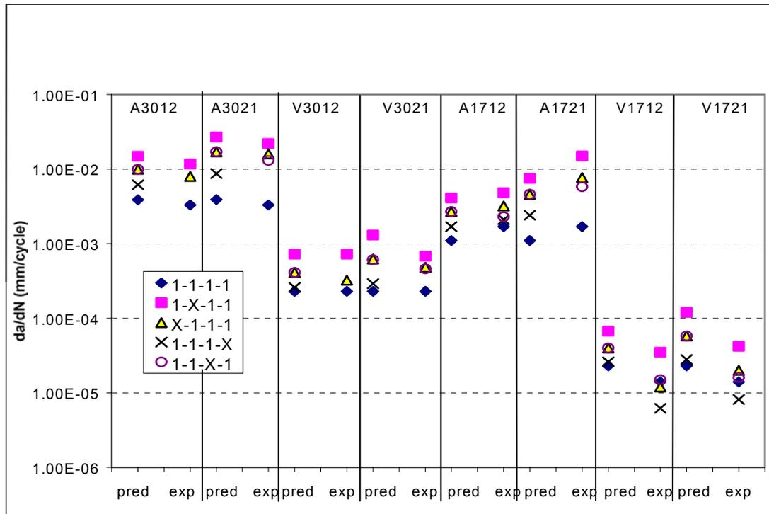
Figure 2: Results of variable waveform tests along with predictions from linear summation model as marked at the bottom of the columns. References at the top of the columns refer the air/vacuum,  $\Delta K$  and total cycle period respectively.
