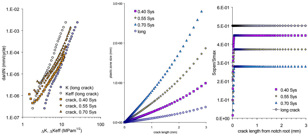
(a) Crack growth rates (b) Crack tip plastic zone sizes (c) Crack opening stresses
