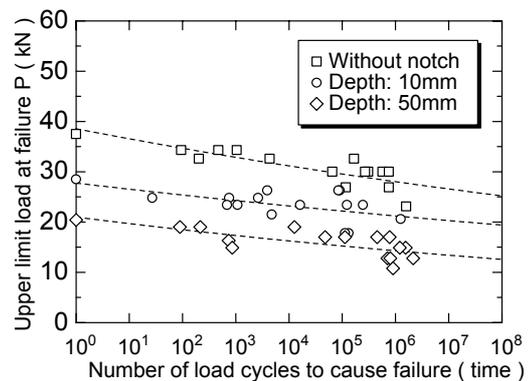
Figure 10: Relation between upper limit load at failure and the number of load cycles to cause failure
