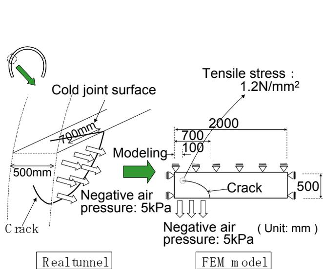
**Figure 11:** Analysis model of the lining of the separation area of the Fukuoka Tunnel
