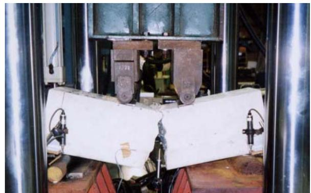
Photo 3: Specimen after failure ( static bend test )
