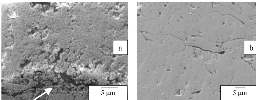
**Figure 1:** (a) Typical microstructure of a nanostructured coating. The white arrow indicates a region where non-molten agglomerated nanostructured particles are observed. (b) Typical microstructure of a conventional coating. The majority of the particles are fully molten.
