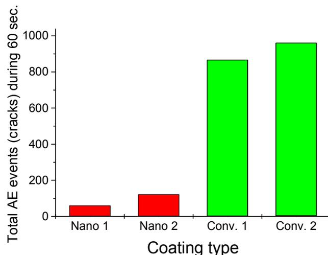
**Figure 2:** Total AE events (cracks) for each type of nanostructured and conventional coatings.
