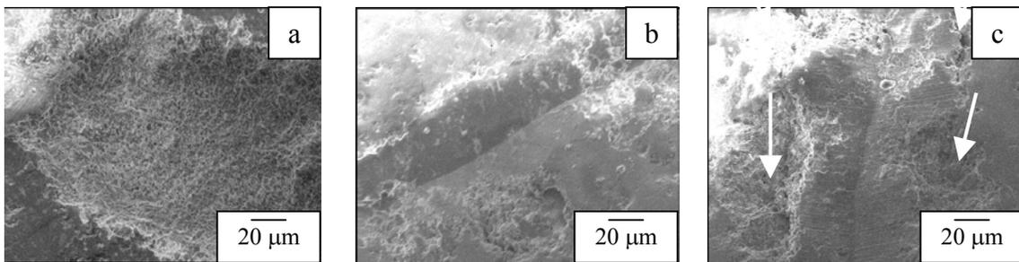
**Figure 3:** SEM pictures of the scar scratch made on nanostructured and conventional coatings. (a) Coating containing 38% of non-molten nanoparticles. (b) Coating containing 23% of non-molten nanoparticles. (c) Conventional coating. The white arrows represent parallel cracks following the scratch scar.
