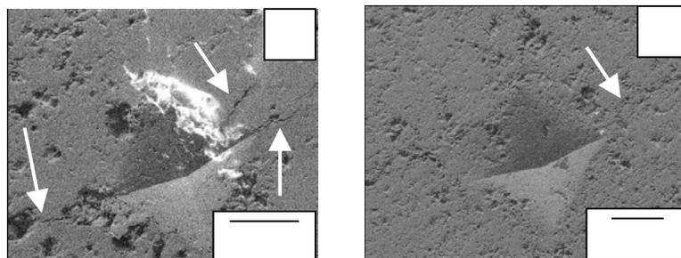
**Figure 4:** Vickers indentation on (a) conventional coating and (b) nanostructured coating. The white arrows are pointing towards cracks.
