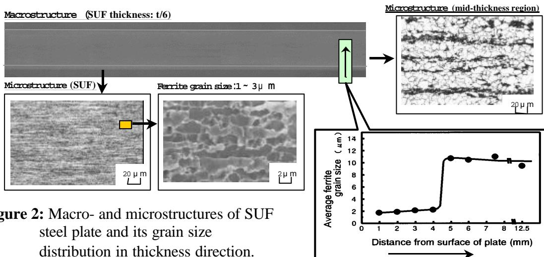
Figure 2: Macro- and microstructures of SUF steel plate and its grain size distribution in thickness direction.
