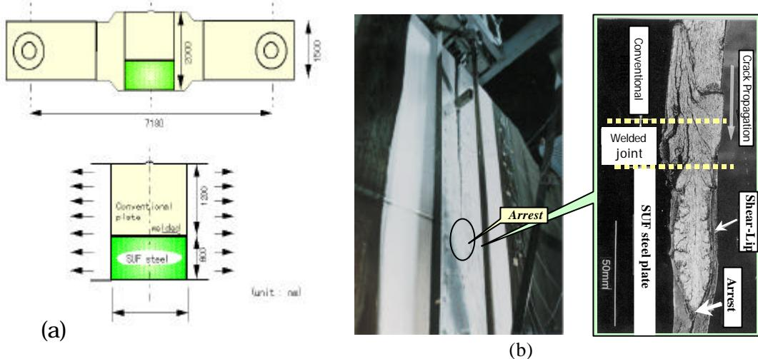
Figure 6: Ultra wide plate duplex ESSO test of SUF steel plate and its fracture surface.
