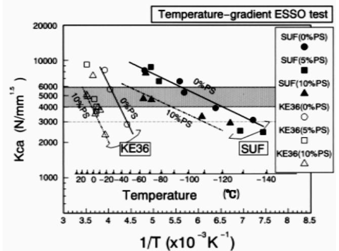
**Figure 4:** Results of temperature gradient type ESSO tests
