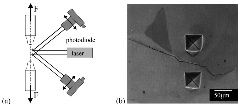
**Figure 1:** Measurement of local displacement by an ISDG system: schematic representation (a) and Vickers microhardness indentations above and below a growing short crack ( $\Delta\sigma/2=600\text{MPa}$   $\updownarrow$ )(b)
