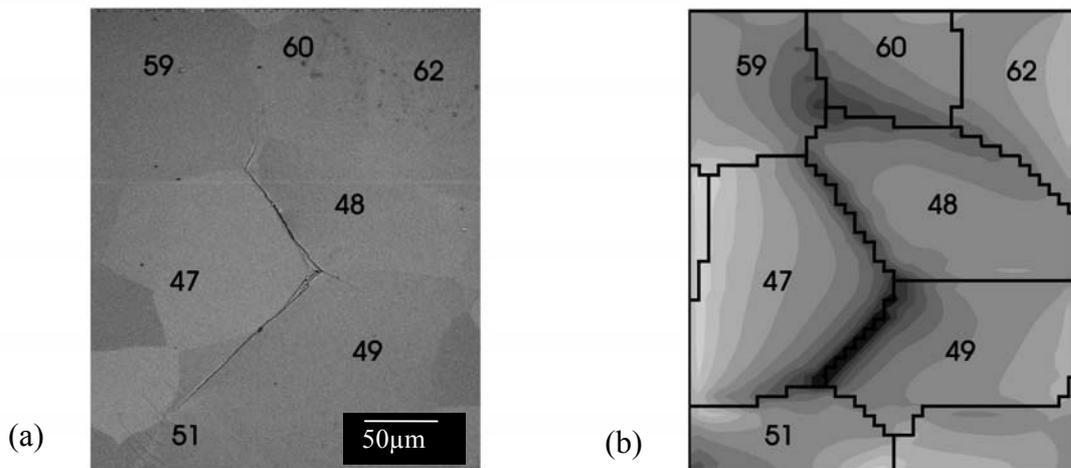
**Figure 3:** Intergranular crack initiation: SEM micrograph (a) and corresponding calculated stress distribution (b) (maximum mean stresses: high stress values = dark) ( $\Delta\sigma/2=600\text{MPa} \Leftrightarrow$ )
