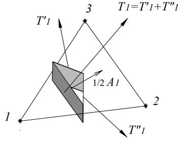
**Figure 4:** Forces acting through the sides of the dual cell of node  $l$ .
