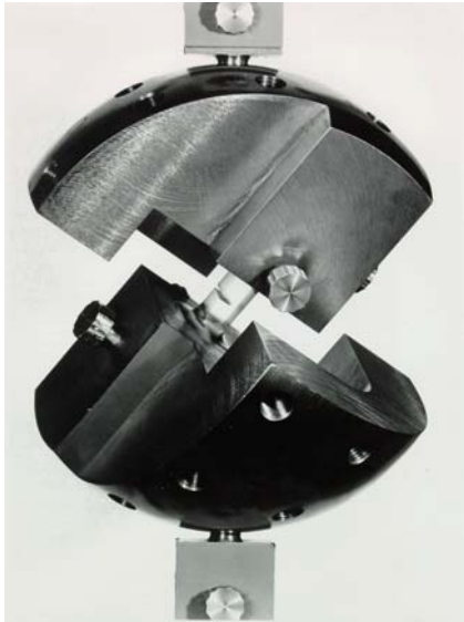
Figure 6: Loading device for the AFM-specimen developed for the superposition of Mode-I+II+III
