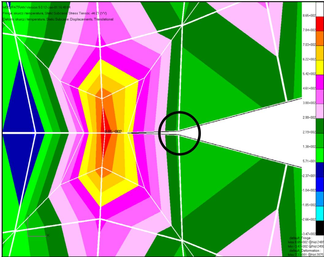
**Figure 2:**  $\sigma_y$  stresses at the crack tip while the load consists of external uniaxial tension, temperature decrease  $\Delta T = -1500$  and the contraction of the macroscopic environment. The crack tip is still opened due to the external uniaxial load (the scale for displacements: 30:1).
