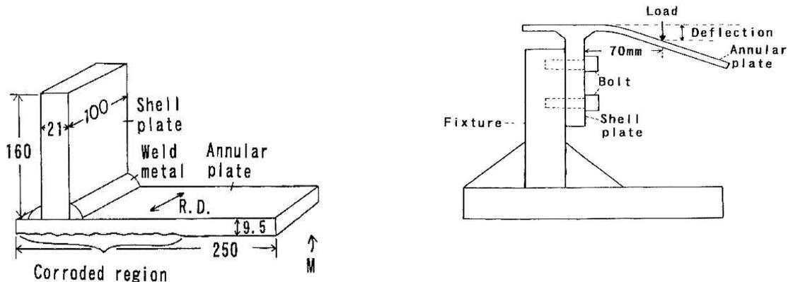
Fig.1. Geometry of L-shaped bend specimen. Fig.2. Schematic illustration of setup for bend test (dimensions in mm).
