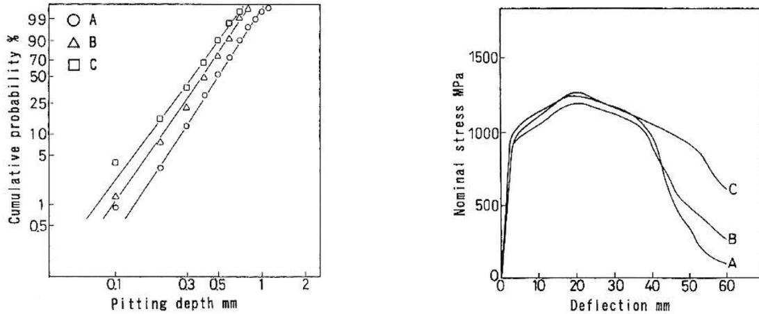
Fig.3. Weibull distributions of pitting depth for specimen A, B and C.
