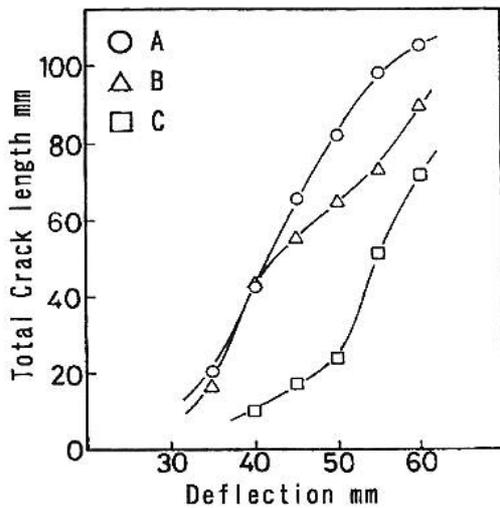
Fig. 9. Relation between total crack length and deflection.
