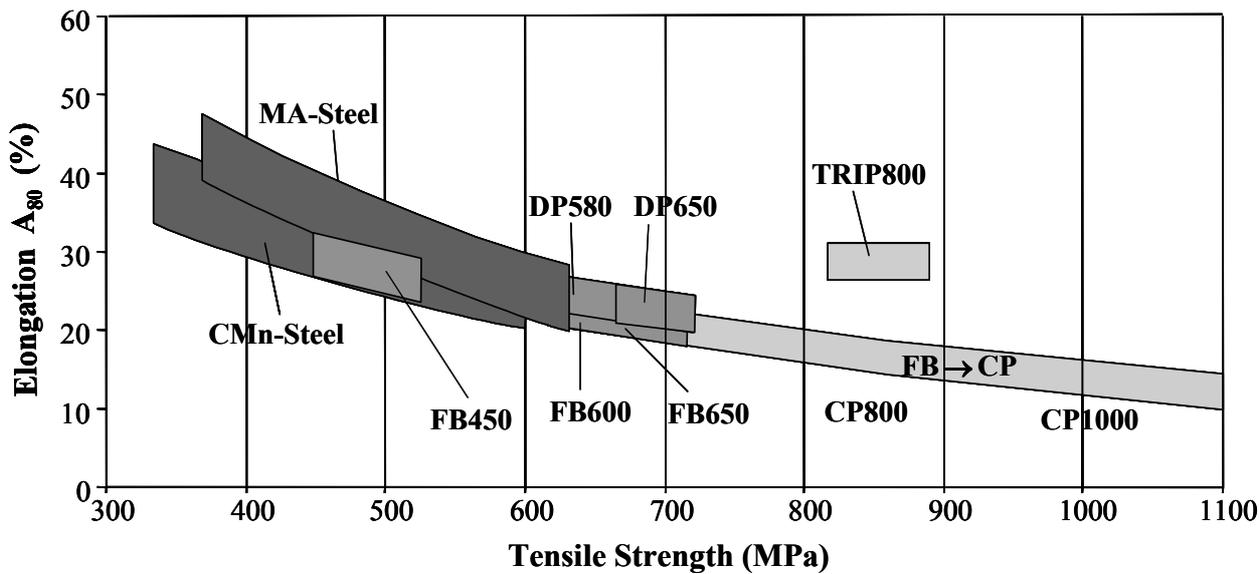
**Figure 1:** Schematic overview of TS and A80 of hot rolled carbon steel products
